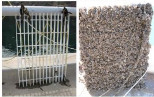
Figure 1 Marine biofouling. Coated steel grate after 9 months of exposure (left image) and uncoated steel grate after 7 months of exposure (right image) [20].
