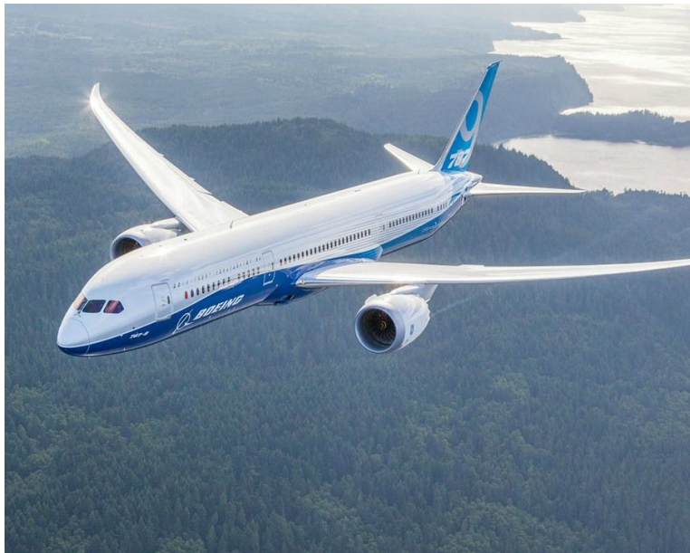
Figure 1. This photograph shows one of Boeing's newest airliners, The 787 Dreamliner, which is an excellent example of a traditional cantilever aircraft which has been made more efficient through the use of lightweight composites and improvements in engine technology. (Johnsson, 2016).
