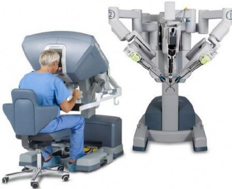
**Fig 2.** The image above shares the common setup for robotic surgery, with the surgeon site on the left and the patient site on the right. The figure also shares the performance-enhancing tools provided by the surgical robot to help the surgeon perform complex endoscopic procedures with relative ease (Nuzzi and Brusasco, 2018).
