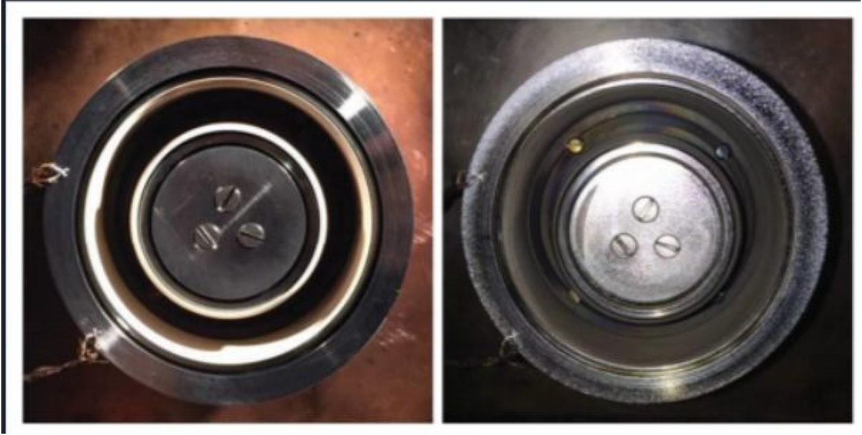
Fig. 3: Above two images show the respective before and after images of a <20 hour long operation test on the MaSMi Miniature Hall Thruster.
