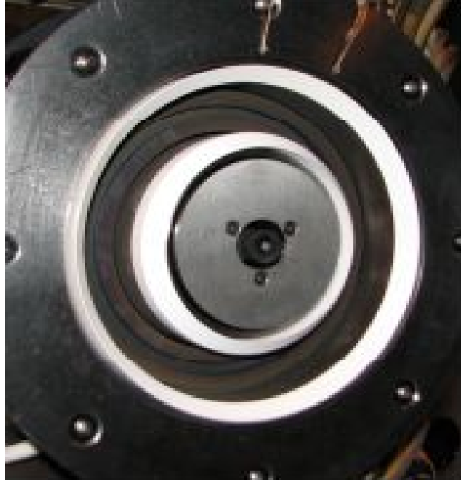
Fig. 6: An image of an H6 with conductive graphite walls.
