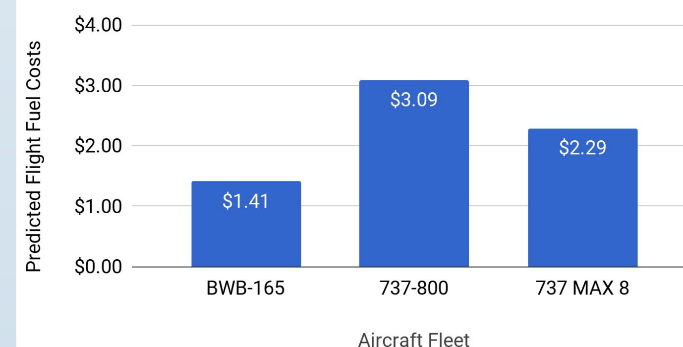
Comparative Fuel Costs for Southwest Airlines Between the BWB-165, Boeing 737-800 and the Boeing 737 MAX 8 Using 2017 Statistics
