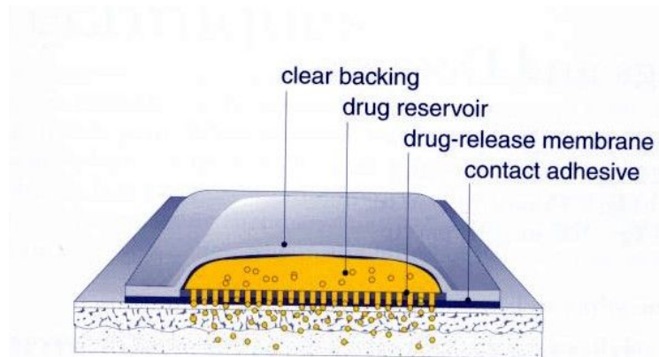
Figure 3. Diagram of the parts of a transdermal patch, developed in the first generation of transdermal drug delivery systems (FDA, 2009).
